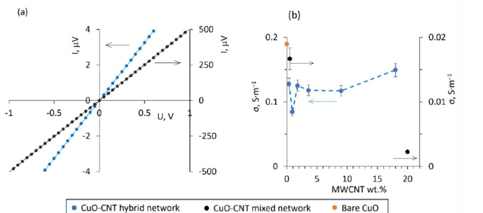
(a) representative current-voltage curves of CuO-MWCNT hybrid composite with ~ 2 wt.% of MWCNTs (blue dots, primary axis) and CuO-MWCNT mixed network with 0.5 wt.% of MWCNTs (black dots, secondary axis); (b) electrical conductivity of bare CuO layer (orange dot), CuO-MWCNT hybrid composites (blue dots), and CuO-MWCNT mixed networks (black dots, secondary axis) vs MWCNT wt.% in the network.
